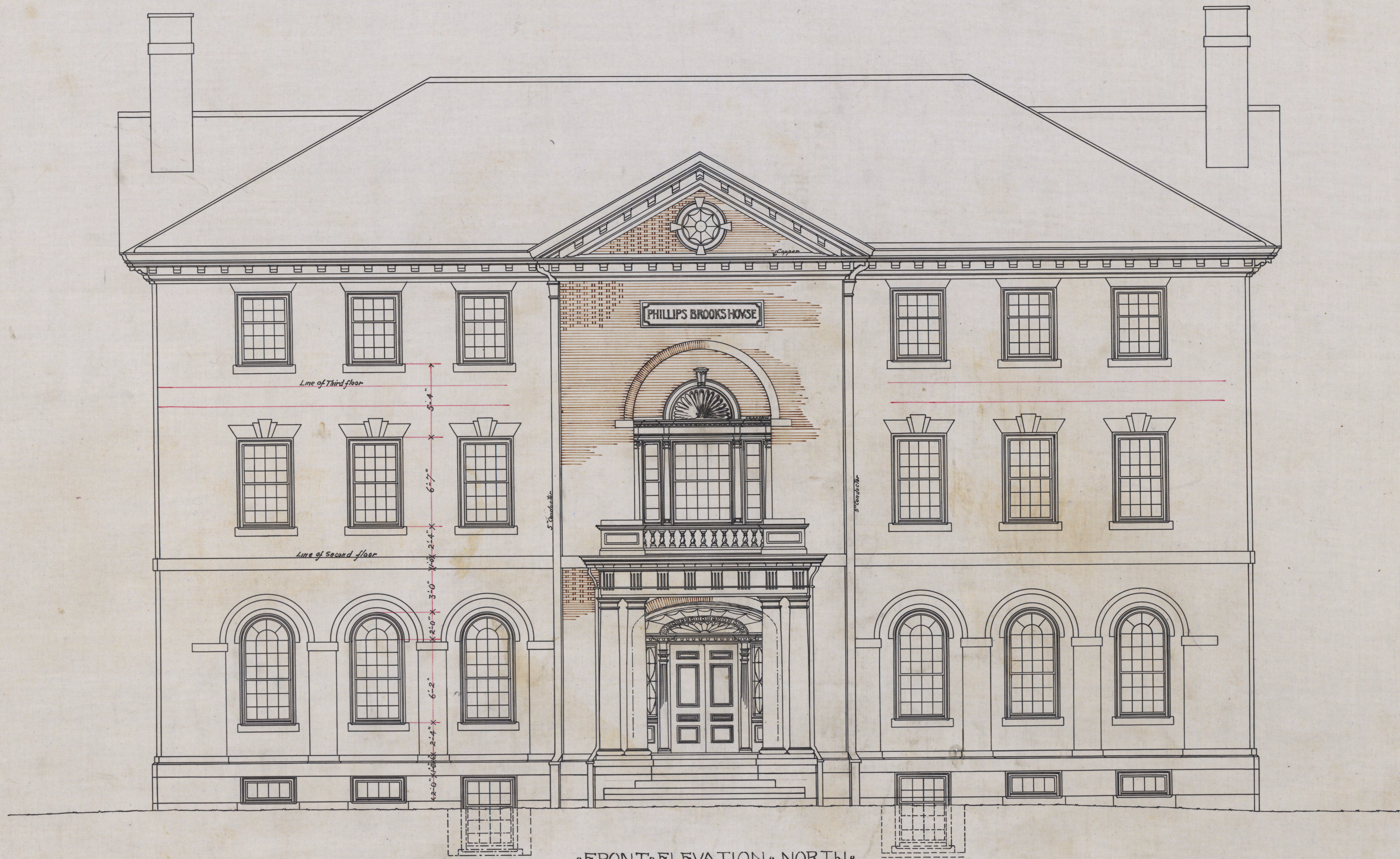
•FRONT•ELEVATION•NORTH• *PHILLIPS* BROOKS *HOUSE* HARVARD *UNIVERSITY* ⑥ •CAMBRIDGE • MASSACHUSETTS • •SCALE • FOUR • FEET • TO • ONE • INCH •
